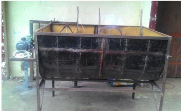
**Gambar 2.** Alat mesin mixer bahan baglog jamur
